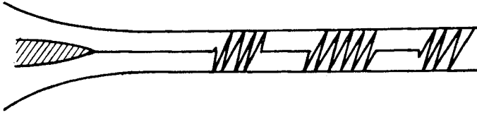
FIGURE 1. The intermittent character of transition as shown by Reynolds.
